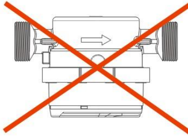
Rys. 2. Prohibited installation positions of water meters manufactured by Apator Powogaz SA, type JS (DN 15-40).
